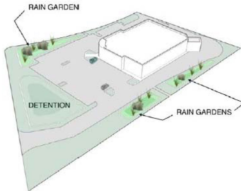
Figure 1.6.7.A-8. Multiple rain gardens may be dispersed across a development, and incorporated into the landscape, providing aesthetic as well as ecological benefits.
